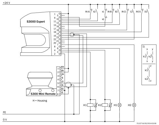
S3000 Expert with S300 Mini Remote in an EFI system with relays/contactors Operating mode: without restart interlock, with external device monitoring
