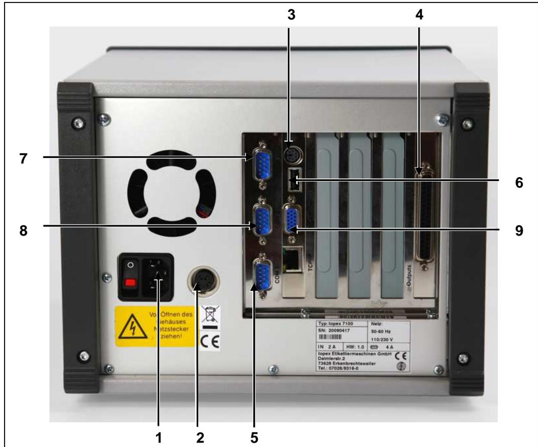
Figure 7 Control unit topex7100 – Rear view
