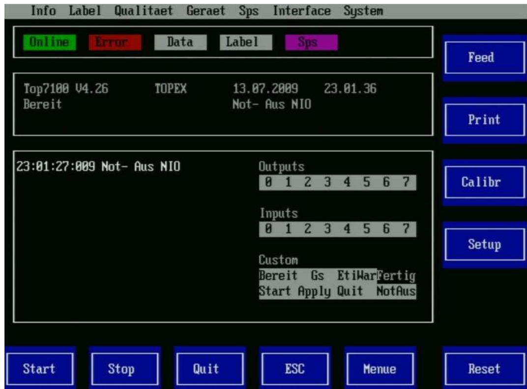
Figure 10 Menu setting of labelling machine
