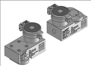
The Access lock HST-TZ1 with an adjacent Actuator serves as access protection and can be used on separating safeguards such as swing doors and sliding doors or flaps. The Actuator can be removed by operating the HST-TZ1, whereby the safeguard
