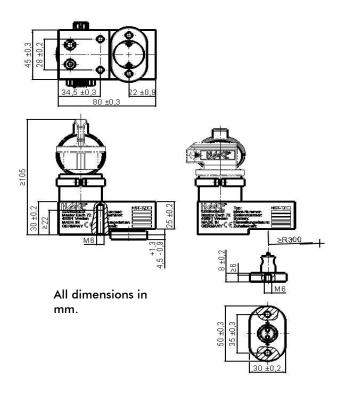
Figure shows a variant of the access lock. The actuator of this variant can be removed from the back. The direction of each variant is listed in the following table.
