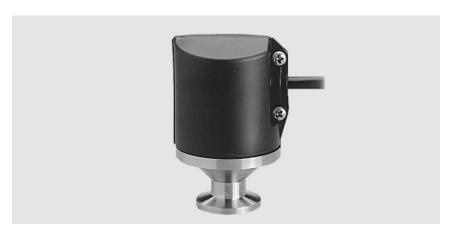
Switch indicating whether or not the pressure has reached the level of the atmospheric pressure after venting. Preset diaphragm pressure switch set to a trigger of 6 mbar (4 Torr) below atmospheric pressure.
