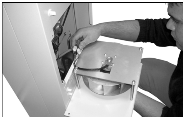
Fig. 65: Disconnect the fan connectors (1)
