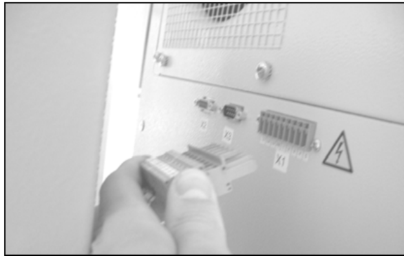
Fig. 53: Disconnect the mains plug
