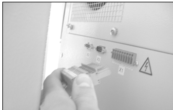
Fig. 34: Disconnect the mains plug
