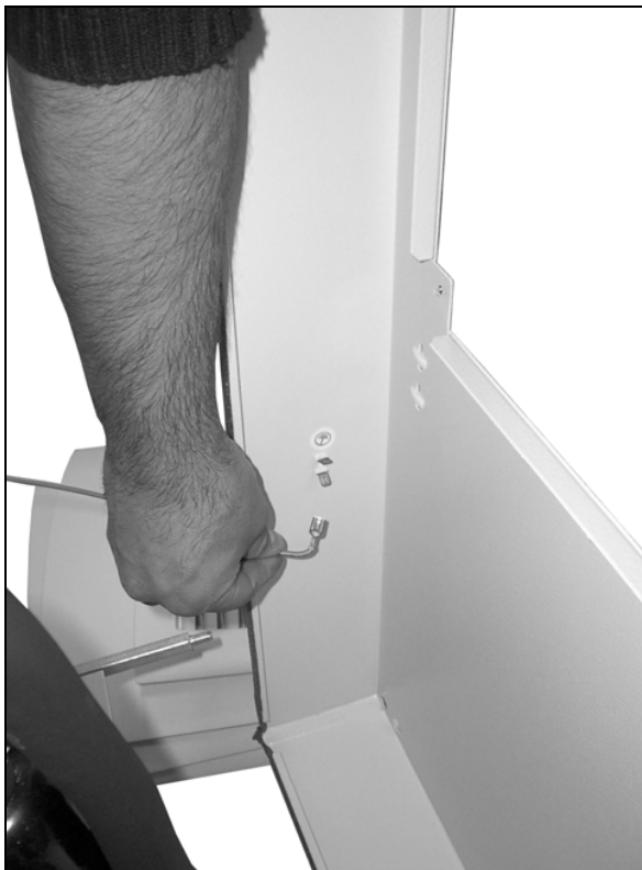
Fig. 73: Disconnect the earthing cable (2)
