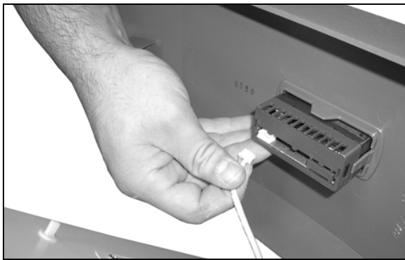
Fig. 60: Disconnect the display cable
