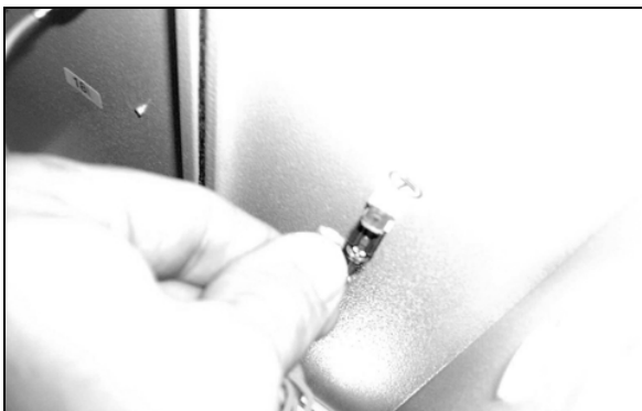
Fig. 69: Disconnect the fan earthing cable (2)
