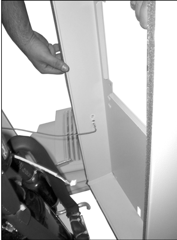
Fig. 72: Disconnect the earthing cable (1)
