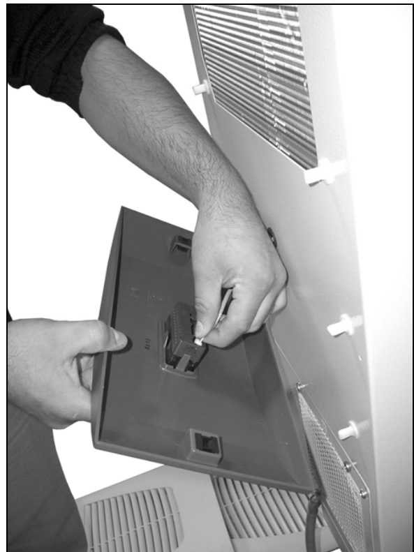
Fig. 38: Disconnect the connector from the display (1)
