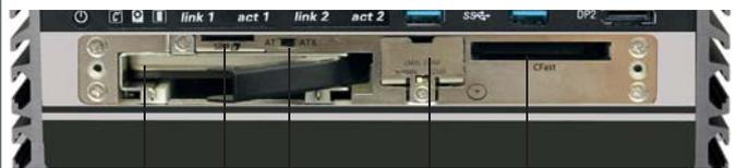
HDD/SSD SIM-Karte AT/ATX Mode CMOS CFast Karte
