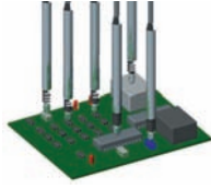
Measuring electronic component dimensions
