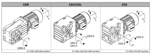
Fig. 2 Direction of rotation of the drive
