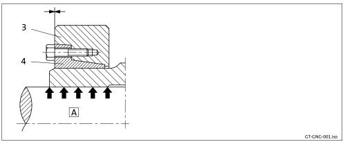
Fig. 9 Hollow shaft with shrink disk
