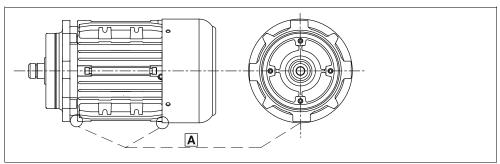
Fig. 14 Motor with condensation drain holes
