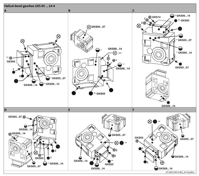
A...F Mounting positions • Oil drain plug
