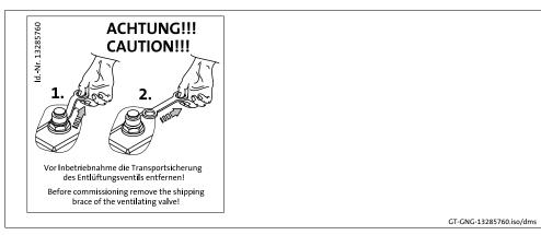
If it deviates from standard mounting positions A - F, the ventilation unit must be checked with regard to its function. Mount ventilation units that are loosely attached (deviating from the standard) as specified in chapter 5.3.11. Gearboxes that are suitable for several mounting positions ( 68) are delivered without ventilation units.
