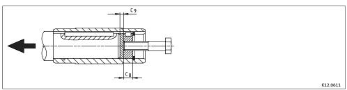
Fig. 6 Disassembly of gearboxes with a hollow shaft, with auxiliary tool; not for GKR
