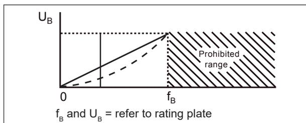
If this is ignored, the motor current will increase disproportionately and the drive motor will fail to achieve its rated speed.
