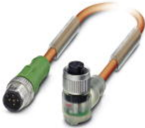
Sensor/Actuator cable, 5-position, PUR halogen-free, Irradiated, orange RAL 2003, Plug straight M12, A-coded, on Socket angled M12, A-coded, with 3 LEDs, Cable length: 1.5 m, Customer-specific version
